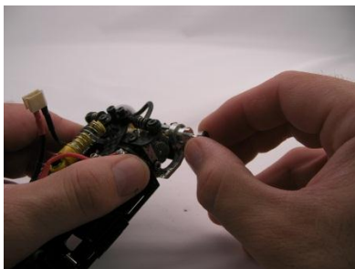
Figure 4- Install 3 x 6 2.5mm bushing/bearing onto diff axle & apply small amount of non-permanent threadlock on diff shaft end
